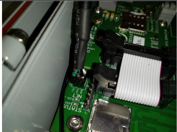
Figure. TTL to USB Connection.
