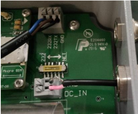
Figure. 110-240VAC to 12VDC@5A Adapter Connection.
